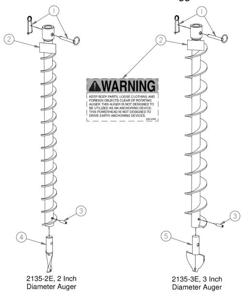
Reference Description Quantity Part Number Number Pin, Auger, .375D 2121 1 1 2 233-5093 Decal, Caution, Clear Rotating 1 3 20051000 Pin, Roll, 5/16 X 1-1/4 1 Bit, Screw, Auger P801 4 1 5 P302 Bit, Screw, Auger
